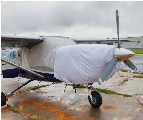
Cessna 207 Engine Cover (test fit)
