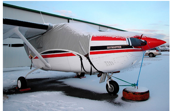
Cessna 337 Skymaster Canopy Cover w/ 14" bib ext., goes back to rear engine inlet and hooks to t.e.
