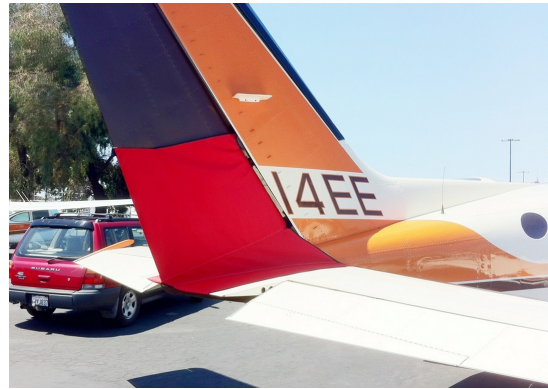
Cessna 414 Rudder Openings Cover (bird barrier)
