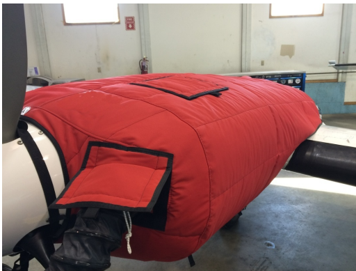
Cessna 402 Insulated Engine Cover with Heater
