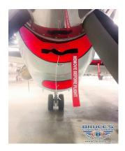
Engine and Oil Cooler Inlet Plugs
