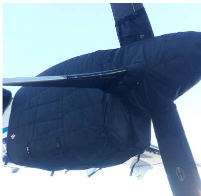
ATR-72-202 Insulated Engine & Prop Hub Covers
