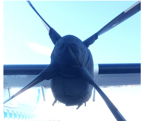
ATR-72-202 Insulated Engine & Prop Hub Covers
