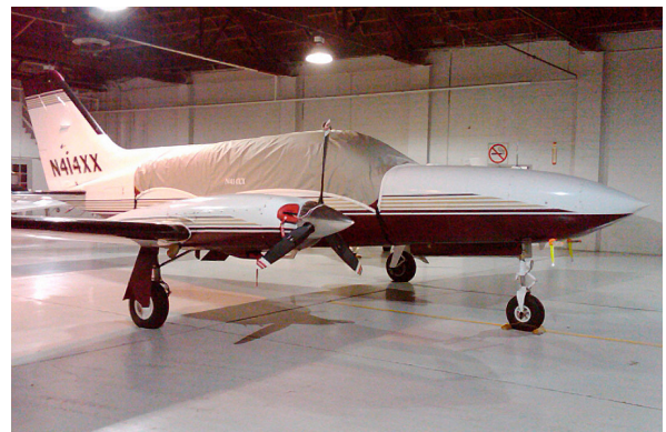
Cessna 414 Canopy Cover and Engine Inlet Plugs
