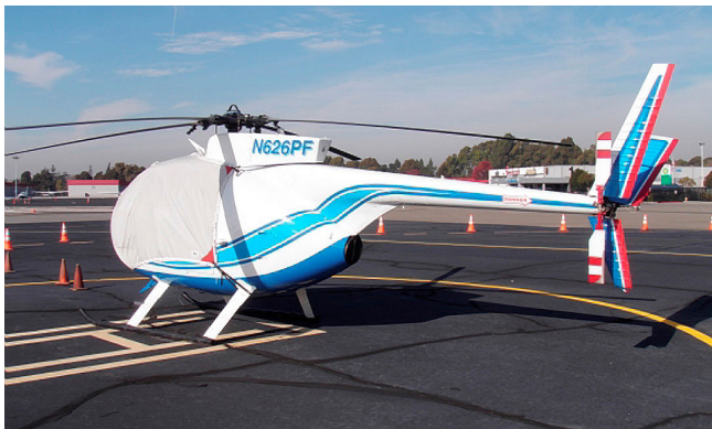
MD500C Bubble Cover with Wire Strike detail
