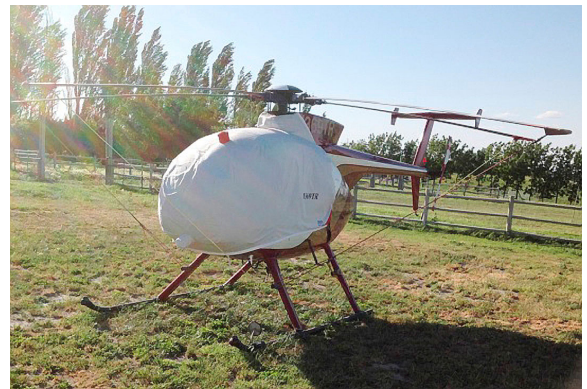
MD500D Bubble Cover with Intake Add-On
