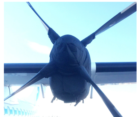
ATR-72-202 Insulated Engine & Prop Hub Covers
