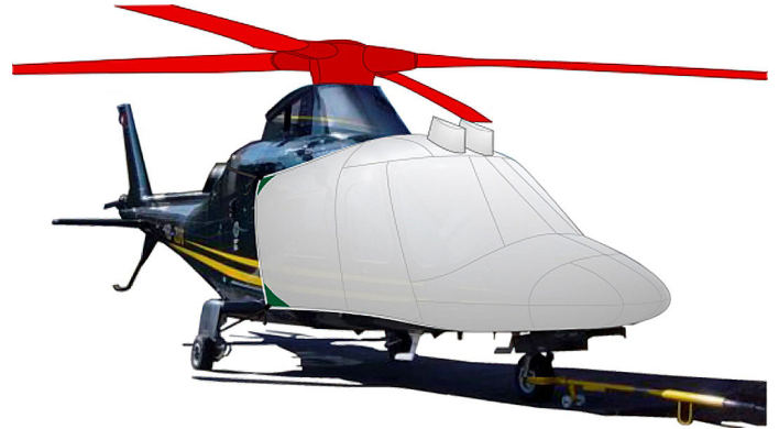
Agusta 109 Bubble, Rotor Hub & Blade Covers (illustration)
