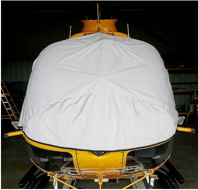
EC-135 Windshield/Skylights Cover, pinches in door jambs
