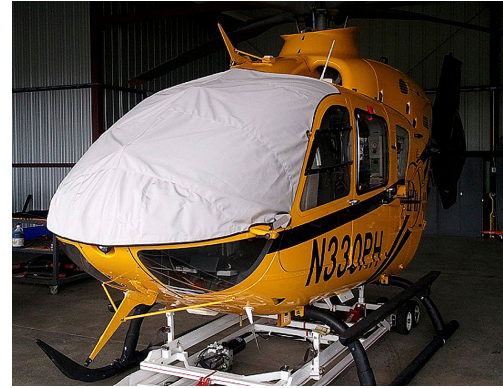
EC-135 Windshield/Skylights Cover, pinches in door jambs
