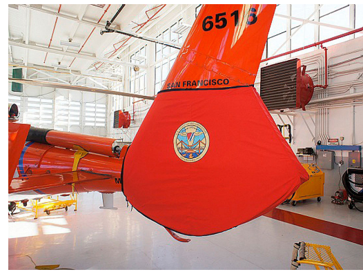
MH-365C Dauphin Tail Fan Fenestron Cover
