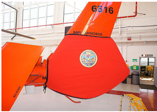
MH-365C Dauphin Tail Fan Fenestron Cover
