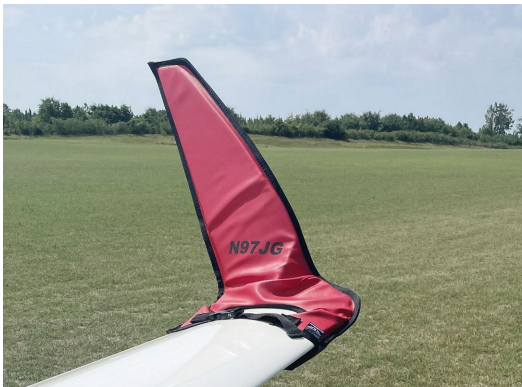
Schempp-Hirth Ventus-2B winglet/wingtip pads
