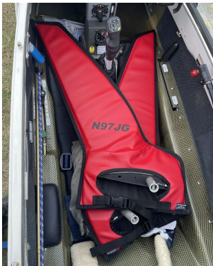
Schempp-Hirth Ventus-2B winglet/wingtip pads
