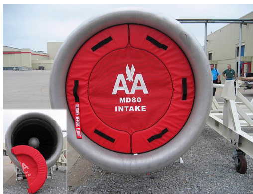
MD-80 JT8D Intake Plug, mesh center & folding type
