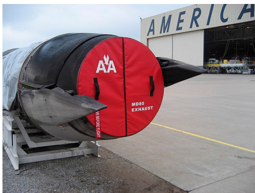
MD80 JT8D Exhaust Plug, Folding Type
