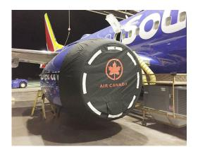
Boeing 737 Intake Cover, CFM LEAP-1B (MAX 7, 8, 9 & 10)
