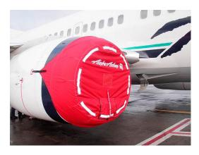
Boeing 737 FOD protection Intake Plug, folding type
