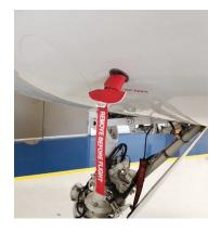
Exhaust Plugs Ship Set, incl. Fan Thrust Reverser and Exhaust Plugs P/N: B767-200
