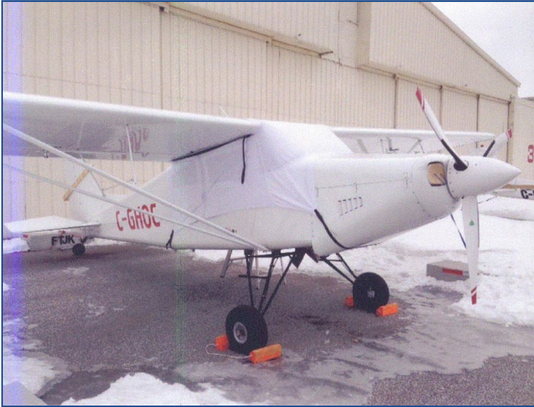
Bushcaddy Canopy Cover, test fit cover
