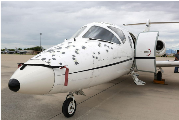
Raytheon Beechjet Hail Damage, and Pitot Covers
