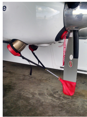
Britten-Norman Islander, prop tie/exh. cover and inlet plug for BN-2T Allison Engines.
