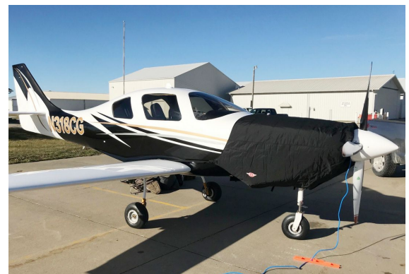
Lancair IV-P Insulated Engine Cover, fully enclosed
