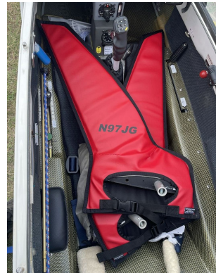
Schempp-Hirth Ventus-2B winglet/wingtip pads
