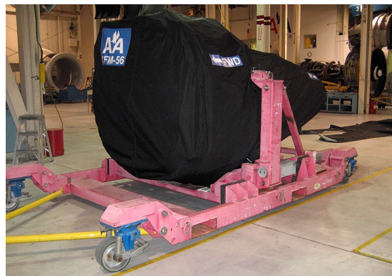
CFM-56-7 Off-link Engine Shipper/Transport cover, w/ Exhaust Cone, fully enclosed
