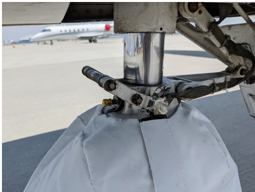
CJ1 Nose Gear Tire Cover, test fit
