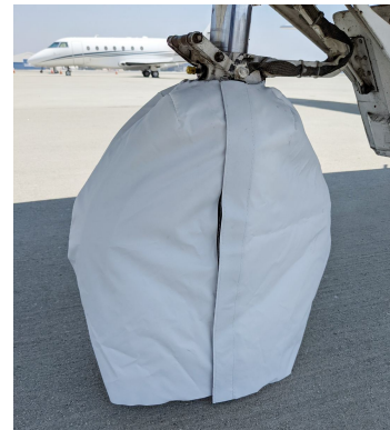
CJ1 Nose Gear Tire Cover, test fit
