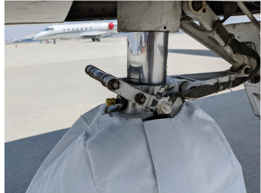
CJ1 Nose Gear Tire Cover, test fit
