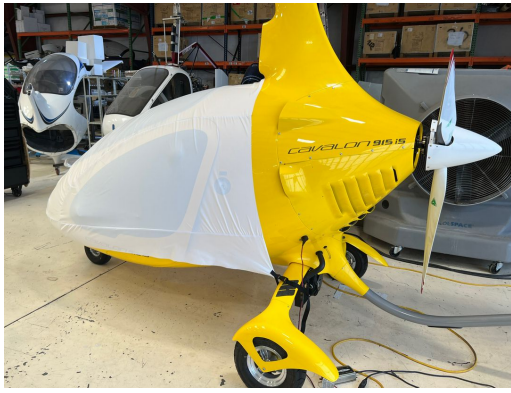
Autogyro Cavalon Canopy/Nose Cover, test fit cover
