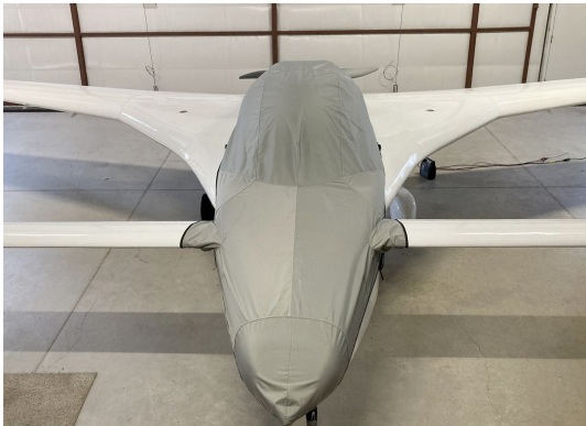
COZY Mk IV Lightweight Travel Canopy/Nose/Engine Cover
