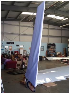
Velocity Vertical Stabilizer Covers, test fit cover
