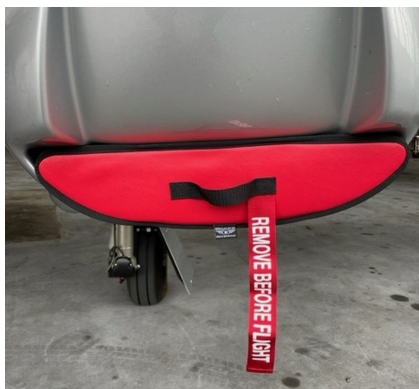
Diamond DA-62 Engine Inlet Plugs ENGINE PLUGS PREVENT BIRD NEST FOD. Piper Saratoga Engine Cowling Bird's Nest
