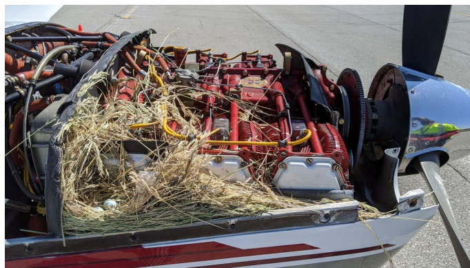
Diamond DA-62 Engine Inlet Plugs ENGINE PLUGS PREVENT BIRD NEST FOD. Piper Saratoga Engine Cowling Bird's Nest
