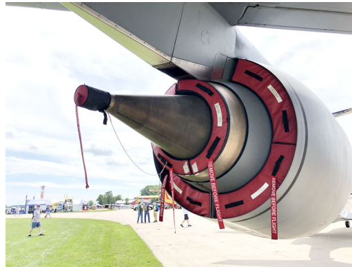
McDonnell Douglas DC-8 Exhaust Plugs, Donut Ring Type For Bypass Vent And Exhaust
