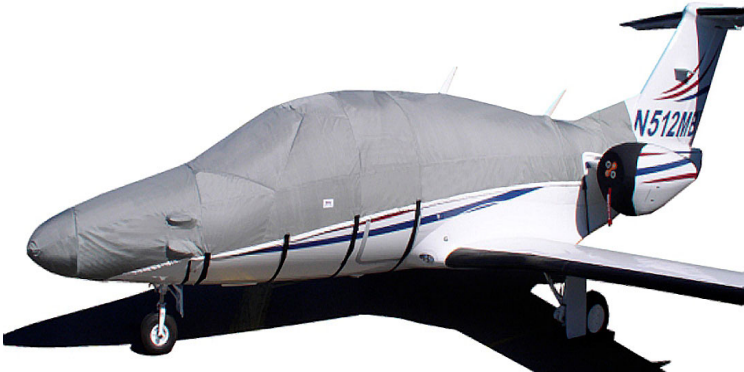
Fuselage Cover, hail protection on all upper surfaces
