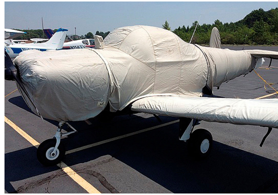
Ercoupe Extended Canopy/Engine & Prop Cover Ercoupe full cover set: Extended Canopy, Engine, Wing & Empennage covers
