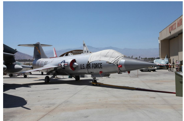
Lockheed F104 Canopy Cover, Intake Plugs
