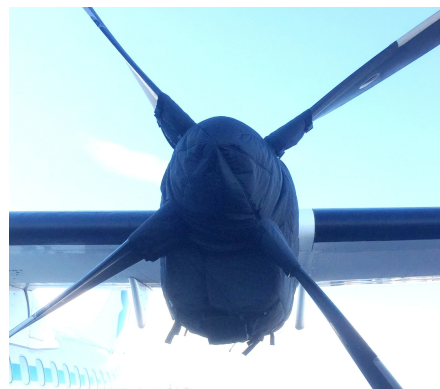
ATR-72-202 Insulated Engine & Prop Hub Covers
