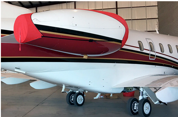
Intake/Exhaust Covers, 3-Strap Type. Successfully installed by two crew, one Challenger 300 Intake/Exhaust Cover Set, 3-strap ladder. type
