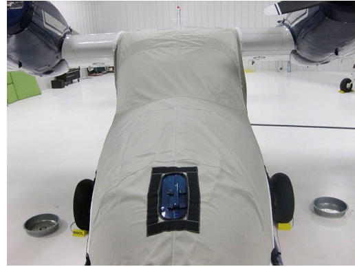
Grumman Widgeon Cockpit/Nose Cover, tie-down cleat detail
