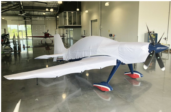
Gamebird GB-1 Extended Canopy/Engine, Wing & Empennage Covers (test fit Game Bird Cockpit Cover, Single Place, 3d model covers)
