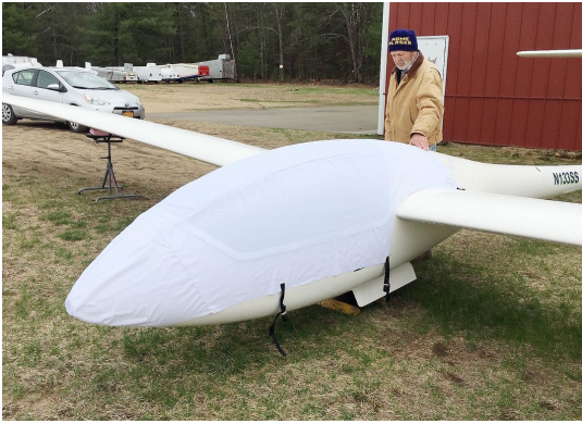
Grob 102 Astir CS Canopy/Nose Cover (test fit)
