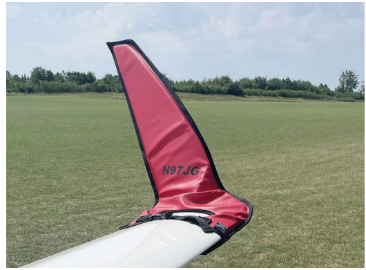
Schempp-Hirth Ventus-2B winglet/wingtip pads
