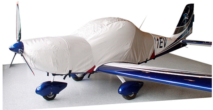
Evekotor Sportstar Extended Canopy/Engine Cover
