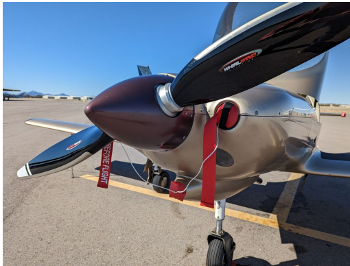
Lancair 320 Engine Inlet Plugs
