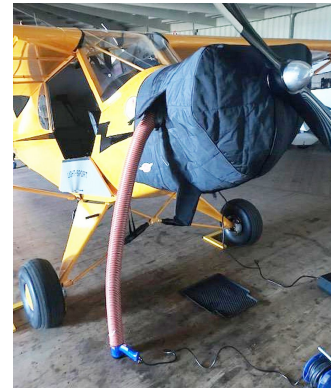
Legend Cub AL3 Insulated Engine Cover with special preheater access vent and attachment detail and fully enclosed under cowling.
