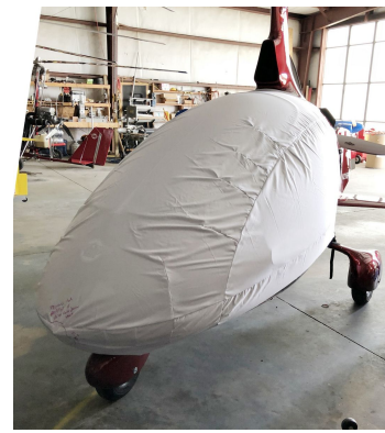
Cavalon Gyrocopter Bubble Cover, test fit cover
