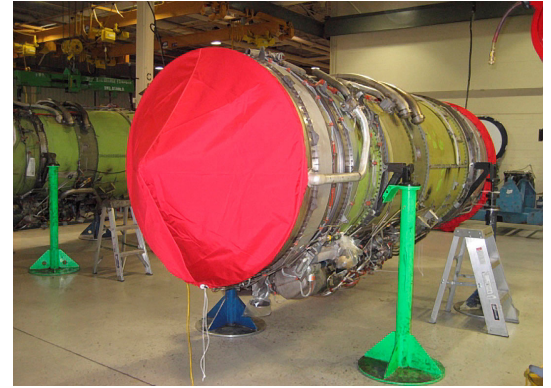
PW JT8D Off-Link Protective Long-term Storage "Rain Cap" Style Engine Cover PW JT8D Off-Link Engine Shower Cap Cover Set
