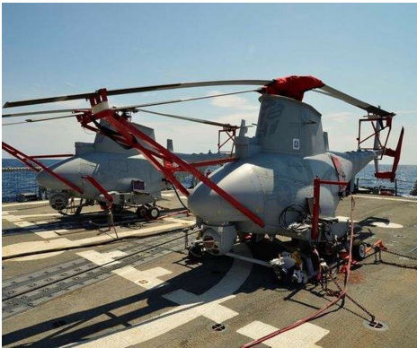
Northrop Grumman MQ-8 Fire Scout Rotor Hub & Tail Rotor Covers
