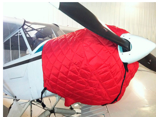
Piper Super Cub Insulated Engine Cover
