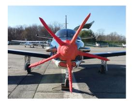
Socata TBM Insulated 5-Blade Prop/Spinner Cover
