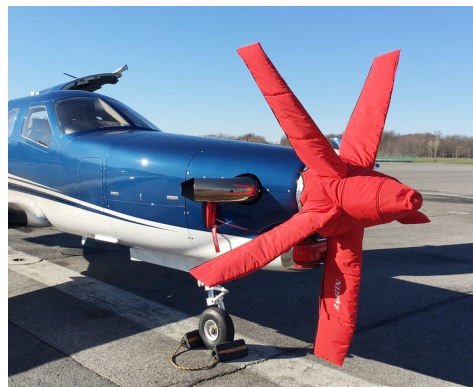
Socata TBM Insulated 5-Blade Prop/Spinner Cover
