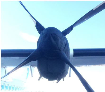
ATR-72-202 Insulated Engine & Prop Hub Covers
