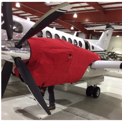
Beech King Air 200 Insulated Engine Cover
