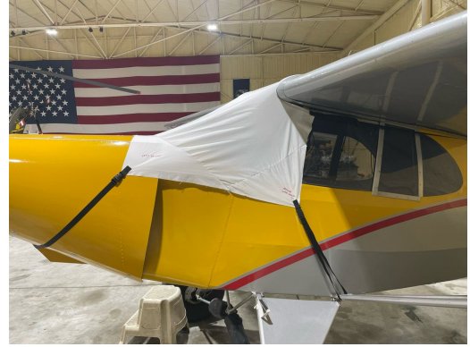
Piper J5A Windshield/Skylight Cover, test fit
