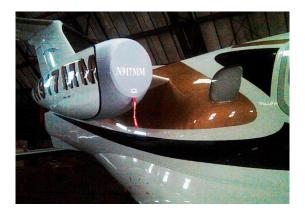
Phenom 100 Intake/Exhaust Cover, "Bikini" Type
