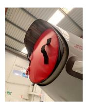
Pilatus PC-24 Engine Exhaust Plug
