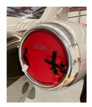
Pilatus PC-24 Engine Intake Plug
