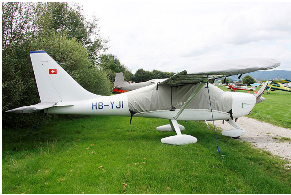
Glstar Canopy, Wings, Horizontal Stab. & Prop Covers
