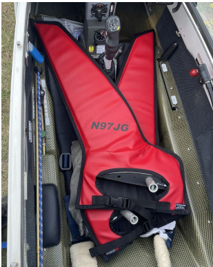
Schempp-Hirth Ventus-2B winglet/wingtip pads
