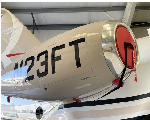
Hawker Beechcraft Premier 390 Intake Plug/Exhaust Plug Set Premier Heat Resistant Pitot Covers set & Engine Intake Plugs
